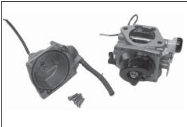
Figure 5-11. Fuel Bowl Removed from Carburetor.
